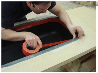
Tape off wall of sink with Karran Protect Plus tape. This prevents solid surface seam adhesive dripping down and bonding to the wall. If that occurs, it can be difficult to remove. A good technique when taping is to overhang the tape by 1/4" then cut the excess off with a sharp blade. Two rows of 2" tape are recommended to protect the top 4" of the bowl walls.
