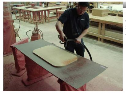
Place sink cutout over the marked area on the back of the laminate. This protects the area where the sink will attach from contact adhesive. Spray contact adhesive.
