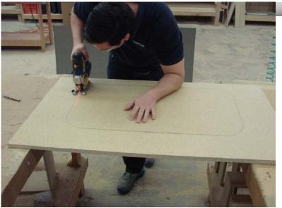
Cut a full width support board. This would be the same dimensions as the front to back dimension of your countertop and about 10" to 12" wider than the sink.
